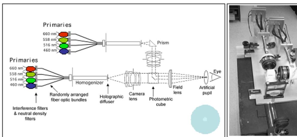
**Figure 4.** The optical setup and a picture of the four primary photostimulator.
